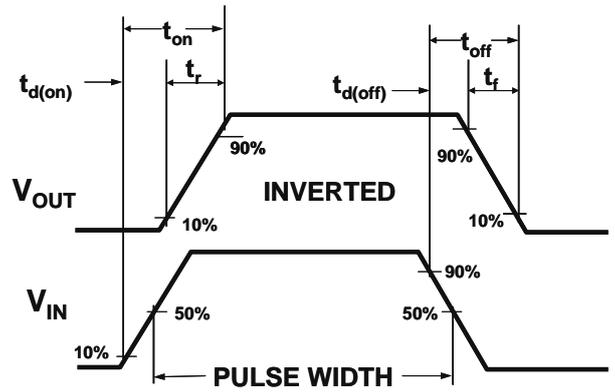
Figure 2: Switching Waveforms
