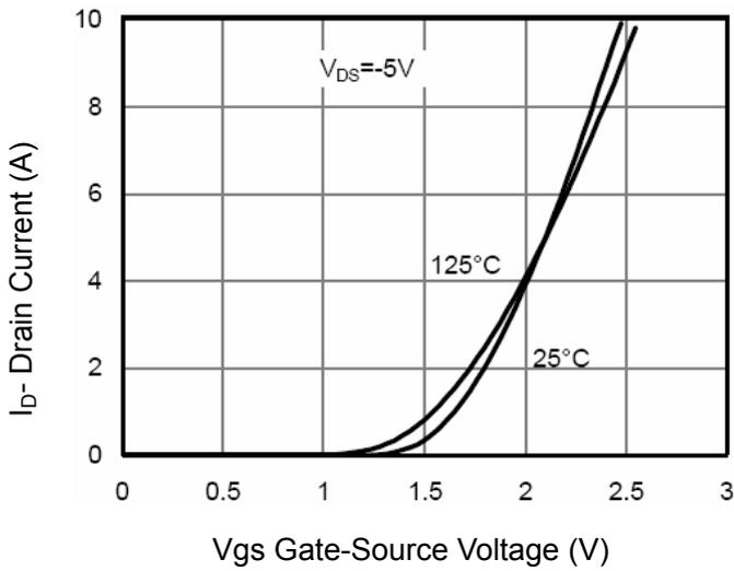
Figure 7 Transfer Characteristics
