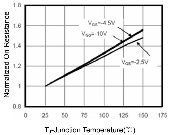
Figure 8 Drain-Source On-Resistance
