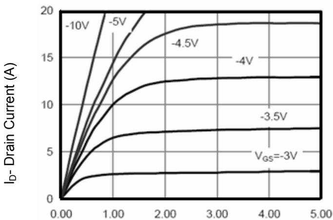
Figure 5 Output Characteristics
