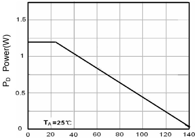
Figure 3 Power Dissipation
