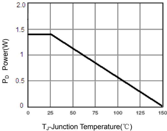
Figure 3 Power Dissipation
