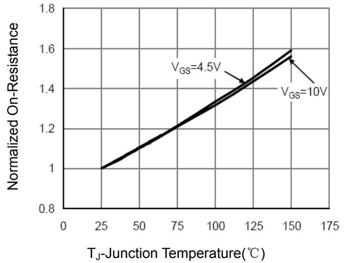
Figure 8 Drain-Source On-Resistance
