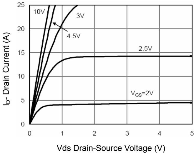
Figure 5 Output Characteristics
