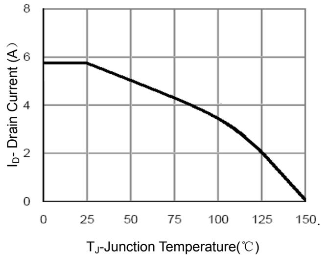
Figure 4 Drain Current
