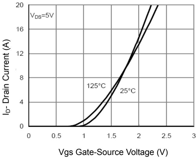
Figure 7 Transfer Characteristics
