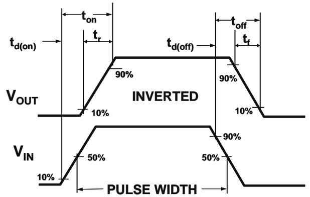
Figure 2: Switching Waveforms
